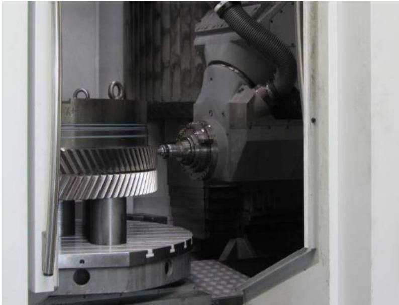
gear milling on 5-axis milling centers
