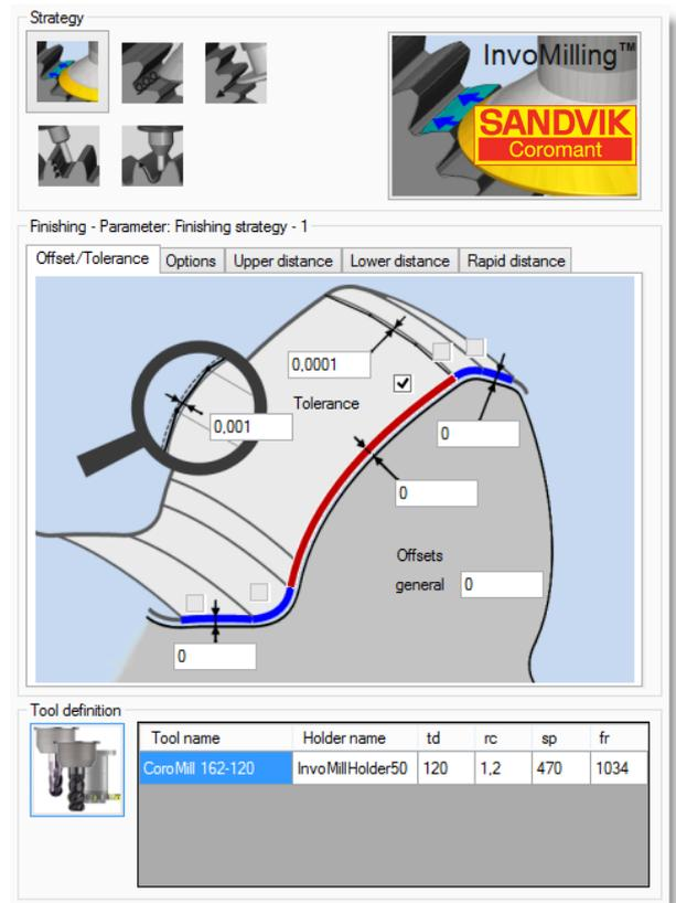
The setup of gear data, tool selection as well as NC programming can be done quickly and user-friendly in **EUKLID GearCAM** and its **InvoMilling™** option.
